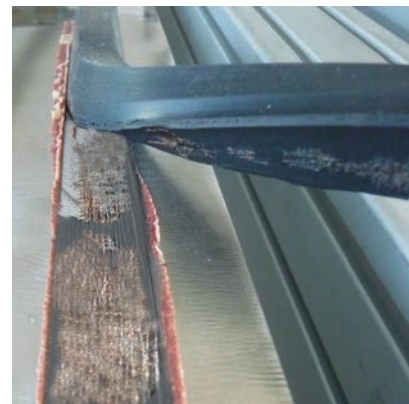
Conventionally bonded v-ropes by other steel belt manufacturers might come loose at temperatures of +176° F (+80° C).
